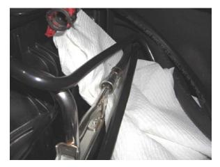
2. Once you have disconnected the OEM female & male fuel lines from one another, connect the Fitch male quick connect to the OEM female quick connect and the Fitch female quick connect to the OEM male quick connect.
