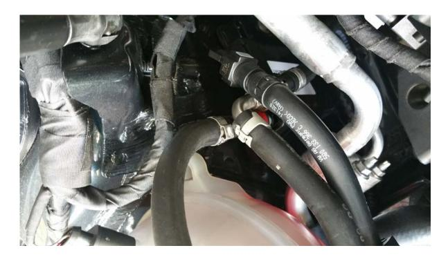
7. Remove the bolt from the engine mount and after putting the Fitch Fuel Catalyst into its mounting bracket then slide the mounting bracket over the engine mount bolt and reattach the engine mount bolt, as the bolt starts to tighten down grab the Fitch and twist it just a bit bending the bracket so that no lines touch anything in the engine bay. Finish tightening down the engine bolt to factory specs.
