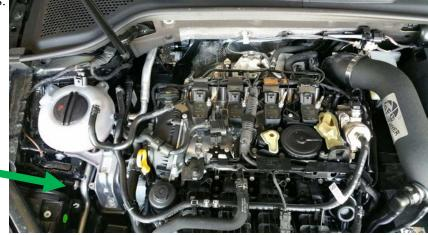
3. Locate the high pressure fuel line in the upper left portion of the engine bay by tracing the line that just was removed from the fuel pump all the way back to the back left of the engine bay.
