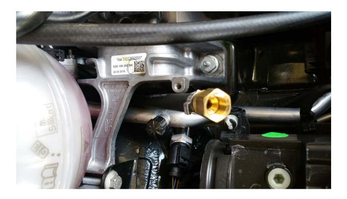
6. Connect the inlet hose of the Fitch to the high pressure OEM hard line, Connect the outlet hose of the Fitch to the stock OEM line that goes across the top of the engine.
