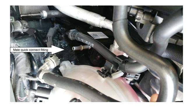
5. Put plastic protection covers over the lines of the Fitch Fuel Catalyst then route the lines between the engine mount and the strut tower brace on the passenger side of the engine bay. Be careful to make sure no exposed line touches the a/c components. (Note: customer may have to supply own plastic line covers or heat tape to wrap the fuel lines)
