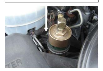
OEM factory male & female fuel supply line quick connect fittings. Adapt to these fittings using the male & female hoses supplied in Fitch kit
