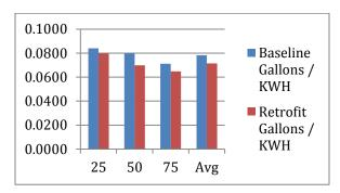
• Dynamometer Test on a Caterpillar 3412
